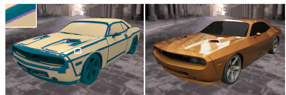
Figure 6: Rendering with a hybrid RBVH – Left: visualization of surfaces represented by height fields (yellow), triangles (green), or both (purple). Right: ray tracing of primary and secondary rays without any visible artifacts.
