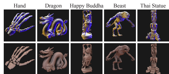
Figure 8: Test scenes listed in Tab. 2 using an RBVH with quality level Q2 for primary (top row) and secondary rays (bottom row); please use the electronic version to zoom in.
